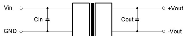
Figure 1: Typical External circuit
